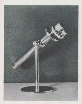
Pocket Polarimeter For ascertaining the concentration of sugar solutions and solutions of optically active substances
