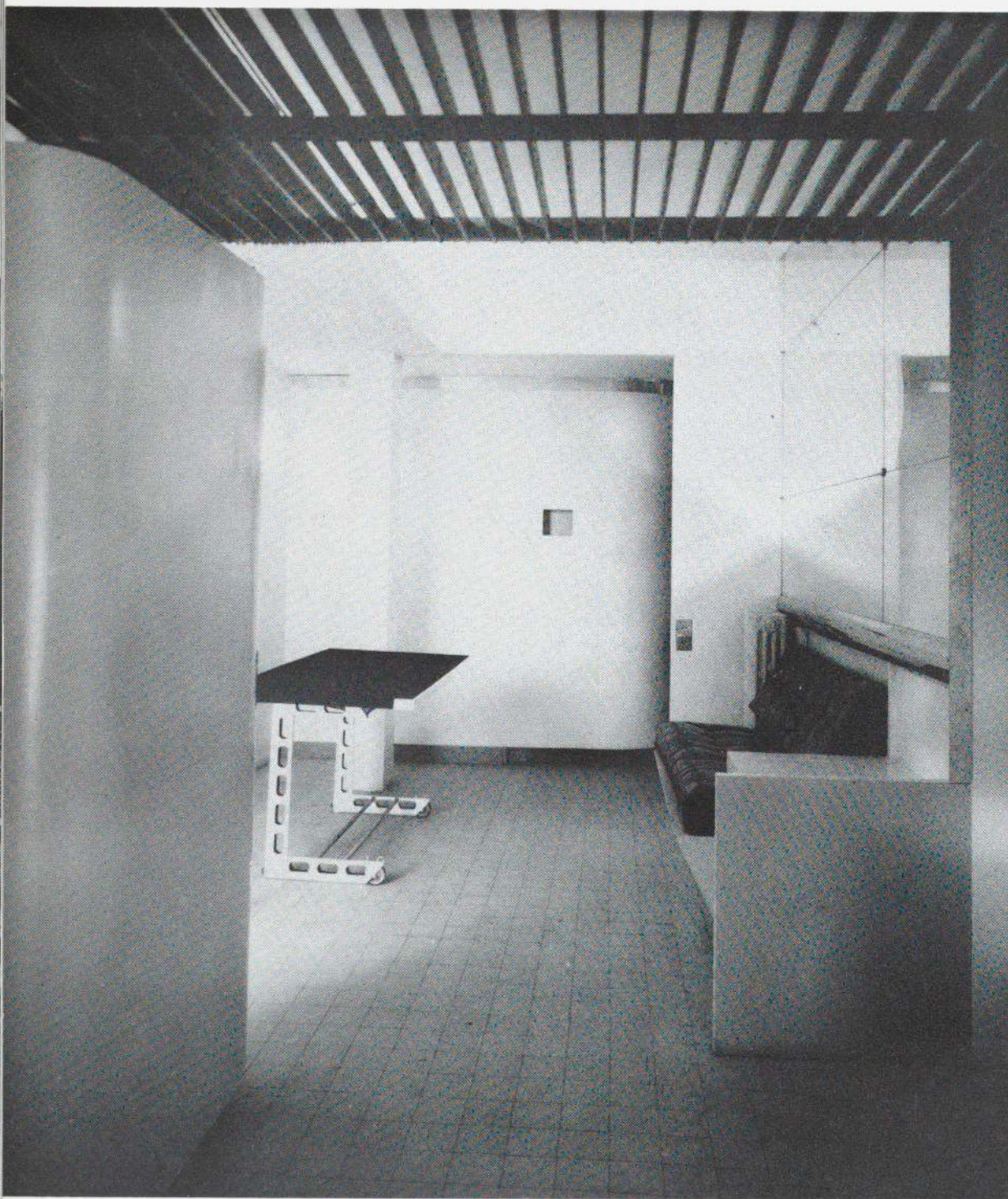
The dining room, seen from the entrance to the studio-living room. The built-in couch, when drawn forward, reveals a narrow staircase leading down into the storage cellar in what had previously been one of the cisterns. The table on its slotted metal base, can be wheeled forward or back.
