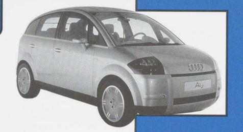
windows supported by light alloy struts. In an attempt to make the car "family friendly," an advanced electronics package includes a steering wheel-based control system, a navigation system, photo-sensors for parking, emergency call, and an automatic distance control that alerts drivers when they are getting too close to the car ahead. A manual gearbox features an automatic clutch.
