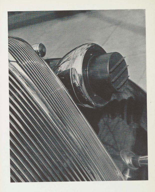
HOODED LIGHT. One of these newly designed headlights must be carried by every vehicle during blackouts.
